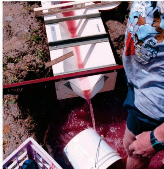
Figure 1. Visual observations with rhodamine WT dye. (A) Spray droplets after drying on peanut foliage. (B) Early raindrops colored by dissolving rhodamine WT. (C) Exposed soil between peanut rows, approximately 10 min after the start of rain; note the deeper dye color on the soil near plants in areas protected from rain. (D) Rhodamine WT color in runoff water, observed throughout runoff event.
